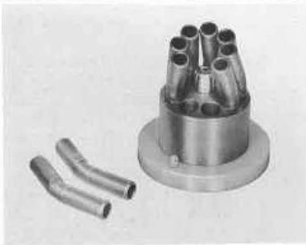
Figure 9 - Assembling Sleeves in Driven Block
