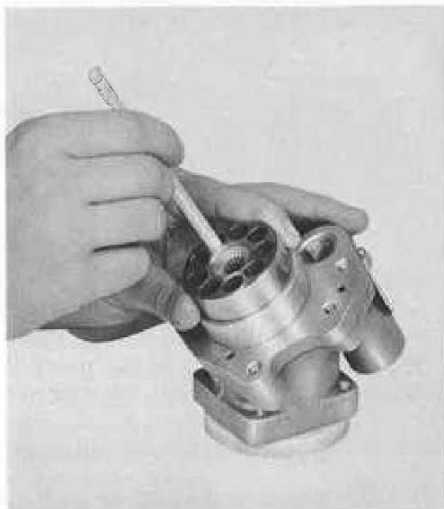
Figure 10 - Aligning the Drive Block and Sleeves
